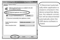
The automatic start of an application is now enabled. When a USB device registered in Meade Virtual Link is connected, the designated application will start automatically.
